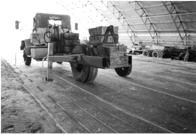
FIG. 10. Test Cart with 13,608-kg Single-Wheel Assembly
